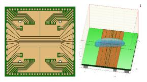
Figure 1 - PCB (left) has current carrying wire structure capable of producing a trapping magnetic potential for the atoms. Simulation (right) shows the resulting shape of the trapped atomic cloud (blue).
